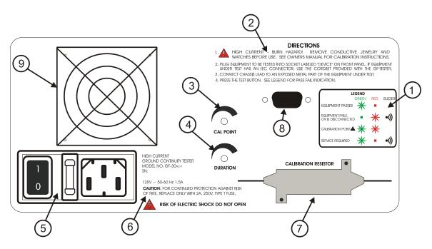
Figure 2-2. Control, Indicators, Connectors - Model GF-30AC-T Rear Panel
